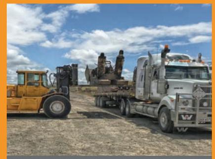
Loading dismantled longwall section to move offsite
