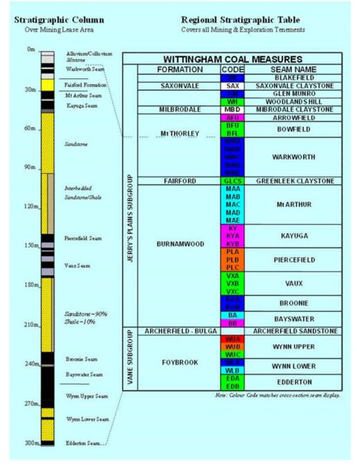
Figure 6: Coal Seam Stratigraphy
