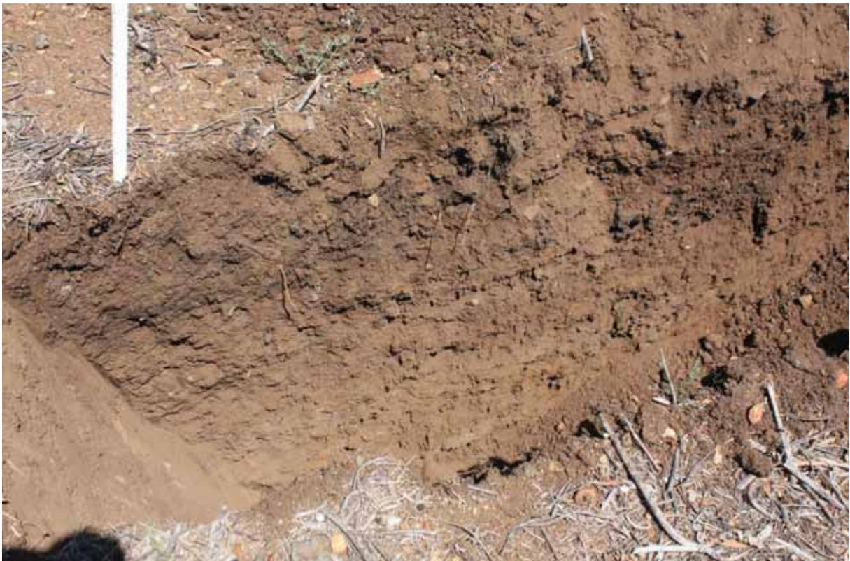
Photo No.2. East Site excavation shows layering of stockpiled material (test pit ET1)
