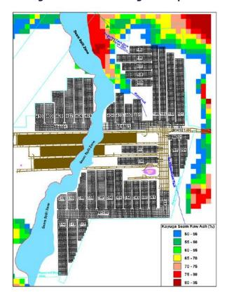
Figure 6 – Plan showing seam split
