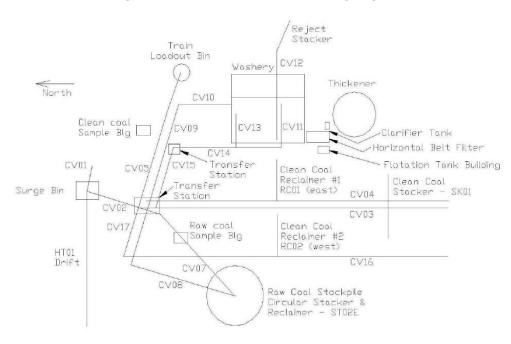
Figure 25 - CHPP Material Handling Layout
