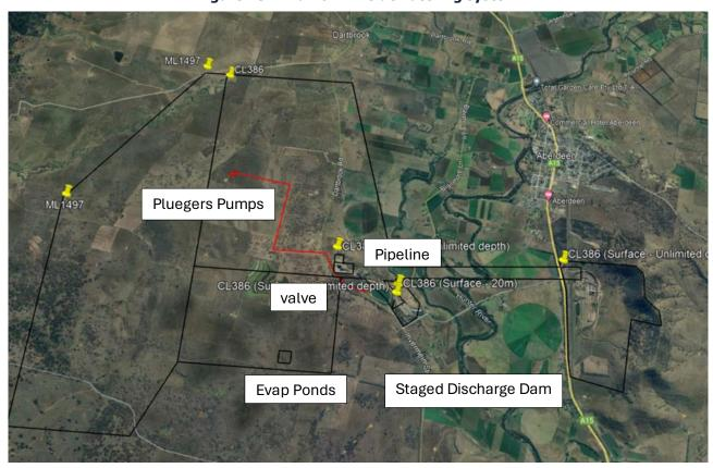
Figure 23 - Plan of mine dewatering system
